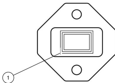
The position of the damping element defined by the positioning system relates to half of the width (center) of the damping element. The measuring range begins and ends with the half coverage provided by the damping element when moving lengthwise.
