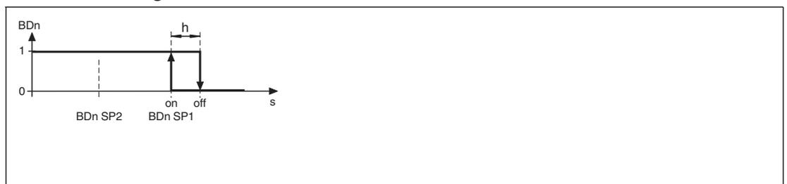
The output switches when the position value is lower than SP1. Any value set in SP2 is ignored.
