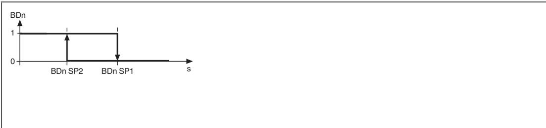
The output switches when the damping element falls below the SP2 position value and switches back when the damping element exceeds the SP1 position value.
