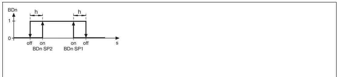
The output switches when an object is between SP1 and SP2.
